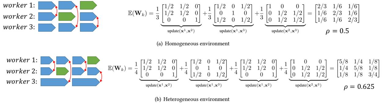
**Figure 4: Illustration of  $\rho$  under different environments. We suppose  $N = 3, P = 2$ , the blue arrow blocks represent an iteration, the green arrow blocks represent the idle time and the red double arrows represent the partial reduce.**
