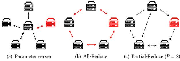
**Figure 1: Illustration of different architectures in heterogeneous environment. The red color represents for the effects from the straggler. The communication manners in partial reduce are adaptively changing in different iterations.**
