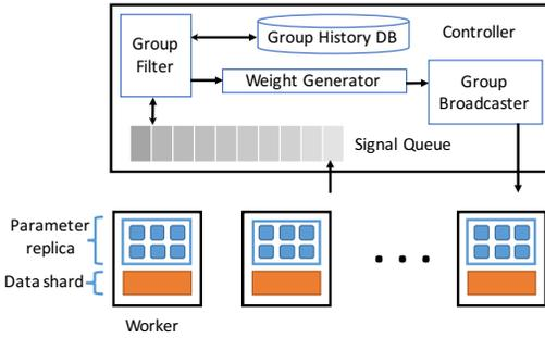
Figure 6: Illustration of the controller architecture.
