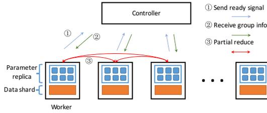
Figure 2: Overview of partial reduce execution.
